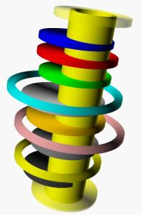
Combining measurement data with design information such as annular ring and drill to copper we can decide if a product meets requirements or if process parameters need to be changed to improve yield/reliability.
